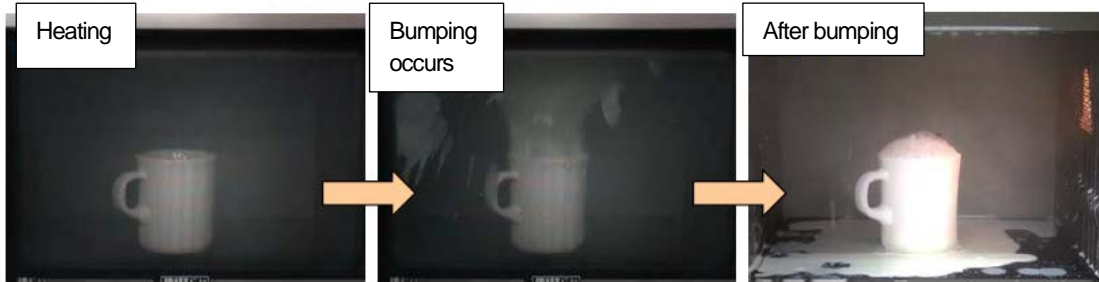
Photo 2. Bumping when soy milk is heated in a microwave oven
