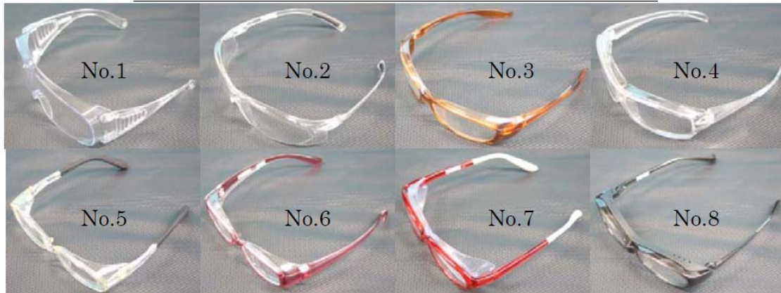
Brands Subjected to Testing (top row: curved type; bottom row: flat type)
